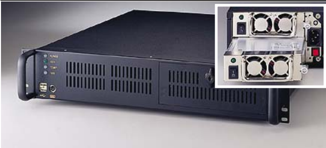
Robust hardware with dual power supply option on 2U models
